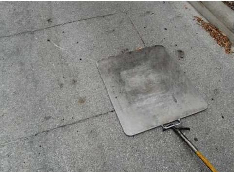
As seen above, the ground pad from the Truck can be slid under the gate with a hook. Once the ground pad is slid into position, the gate will open. As mentioned earlier, it has to go over the induction loop that is the furthest away from the gate.
